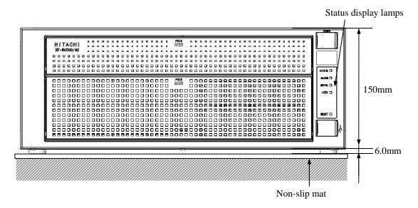
Figure 1-3 Installation Requirements (Horizontal Installation on the Desktop)
