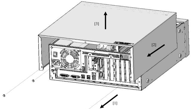
Figure 5-2 Removing the Cover of the Equipment
