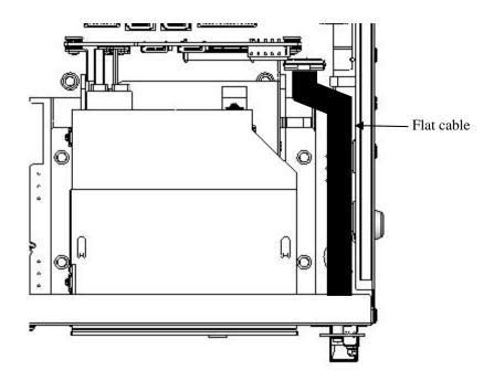
Figure 5-18 Attention about HDD frame connection
