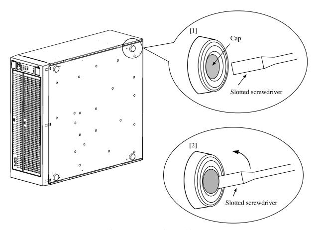
Figure 5-20 Removing a Rubber Foot
