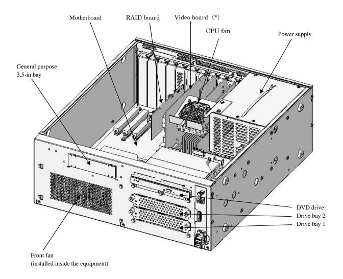
Figure 2-3 (2) Physical Configuration Inside Equipment (D model)
