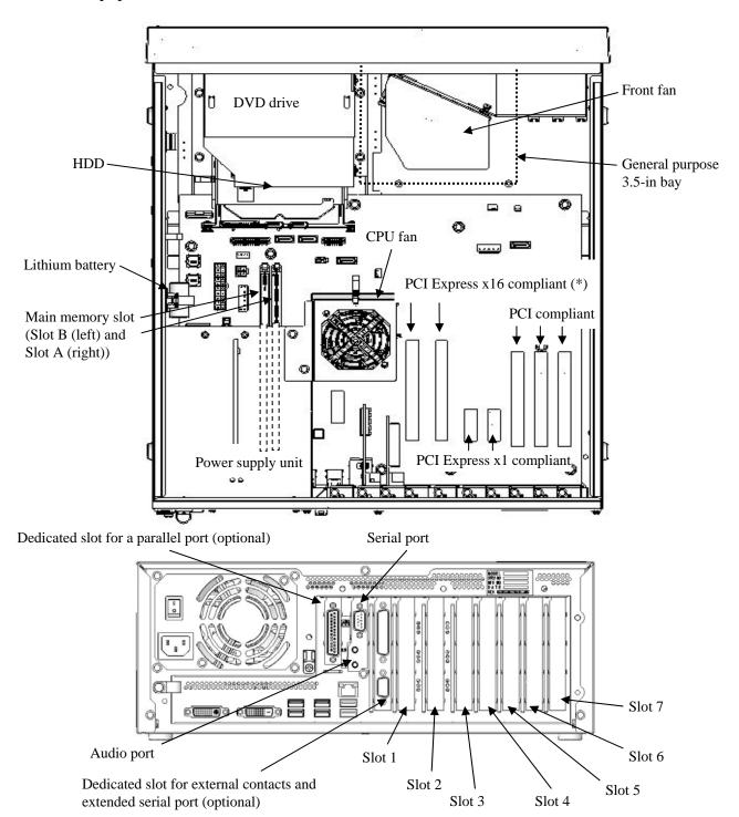
(\*) A PCI Express x16 connector is used but the internal connection is equivalent to PCI Express x8.
