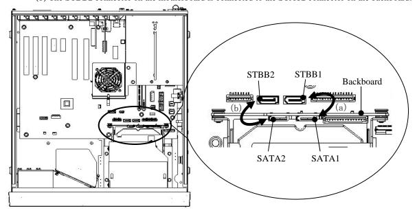
Figure 5-12 Connecting SATA Cables
