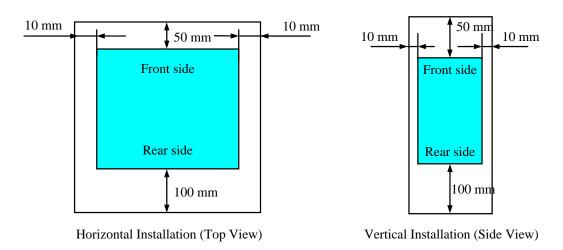
Figure 1-2 Installation Clearance
