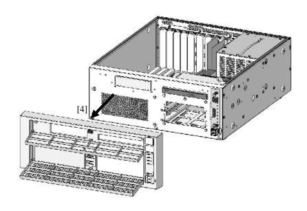
Figure 5-10 Removing the Front Panel
