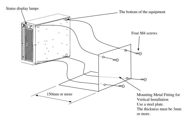
Figure 1-5 Installation Requirements (Vertical Installation on the Desktop)
