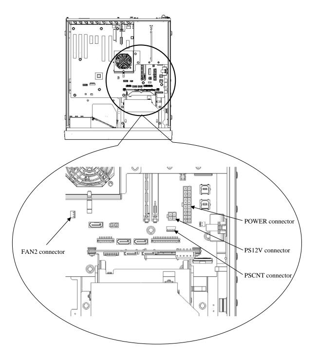
Figure 5-5 Internal Cabling near the Power Supply inside the Equipment
