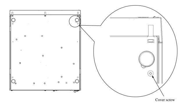
Figure 5-21 Removing Cover Screws
