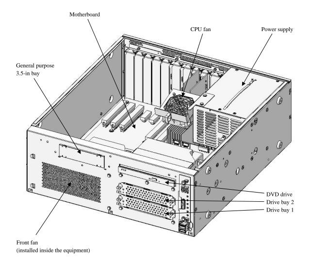
Figure 2-3 (1) Physical Configuration Inside Equipment (A model)
