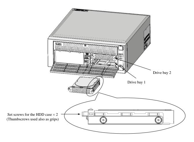
Figure 5-8 Installing and Removing an HDD
