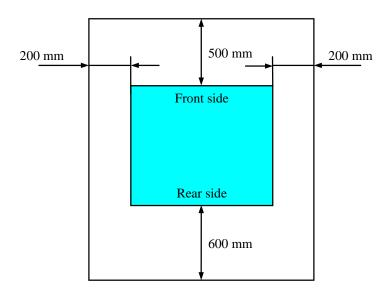
Figure 1-1 Operation and Service Clearance (Top View)
