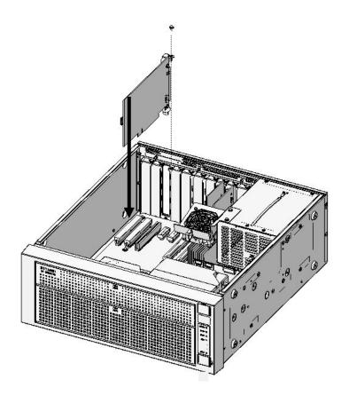
Figure 5-4 Installing an Extension Board
