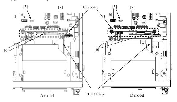
Figure 5-11 Removing Internal Connections
