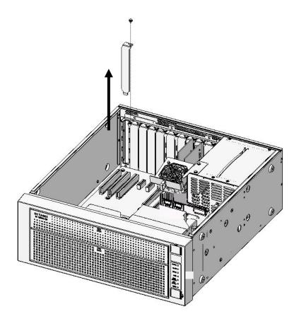
Figure 5-3 Removing a Slot Cover
