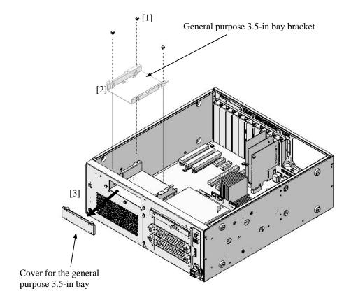
Figure 5-22 Removing the General Purpose 3.5-in Bay Bracket
