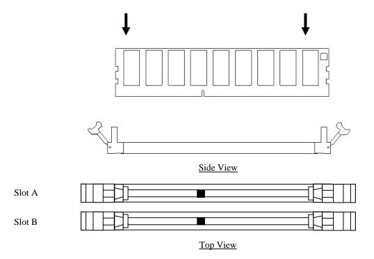
Figure 5-7 Installing Main Memory
