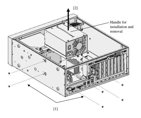
Figure 5-6 Removing the Power Supply
