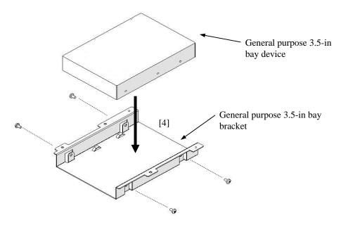
Figure 5-23 Mounting the General Purpose 3.5-in Bay Device
