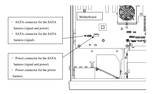
Figure 5-25 Connecting a Harness
