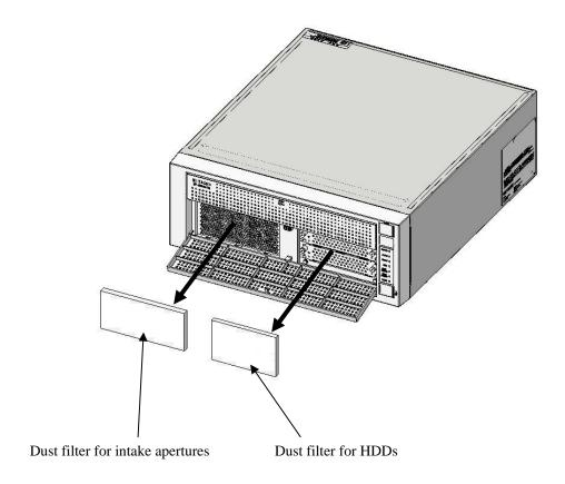
Figure 5-26 Replace a dust filter
