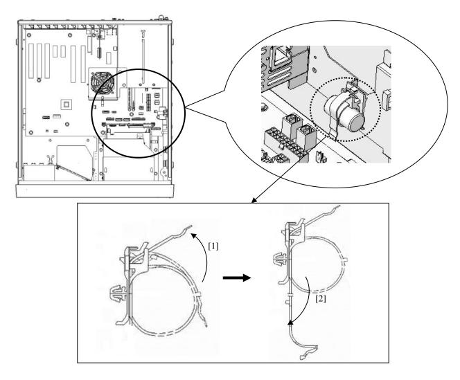
Figure 5-27 Removing the Lithium Battery
