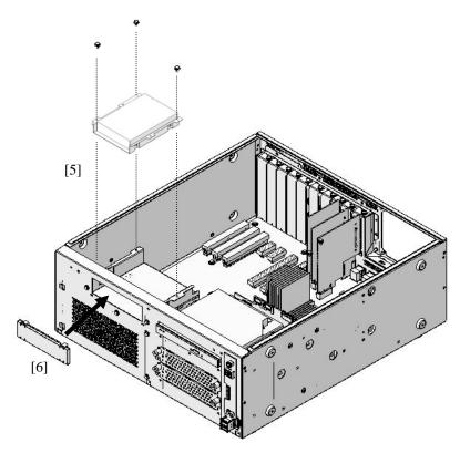
Figure 5-24 Mounting the General Purpose 3.5-in Bay Bracket
