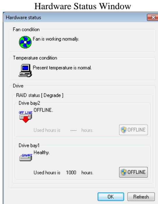
(Note) This window shows that the HDD in drive bay 2 is defective.
