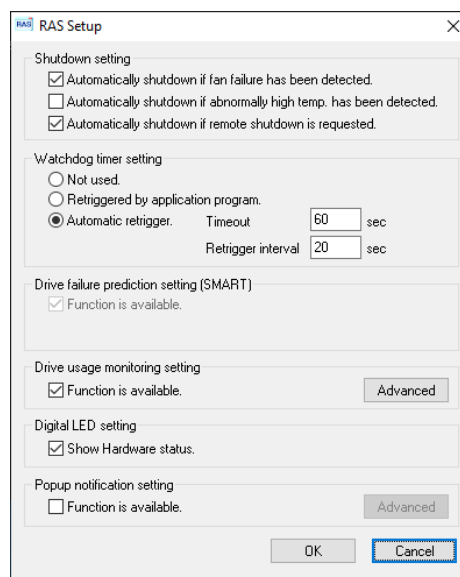
Figure 1-1 RAS Setup Window
